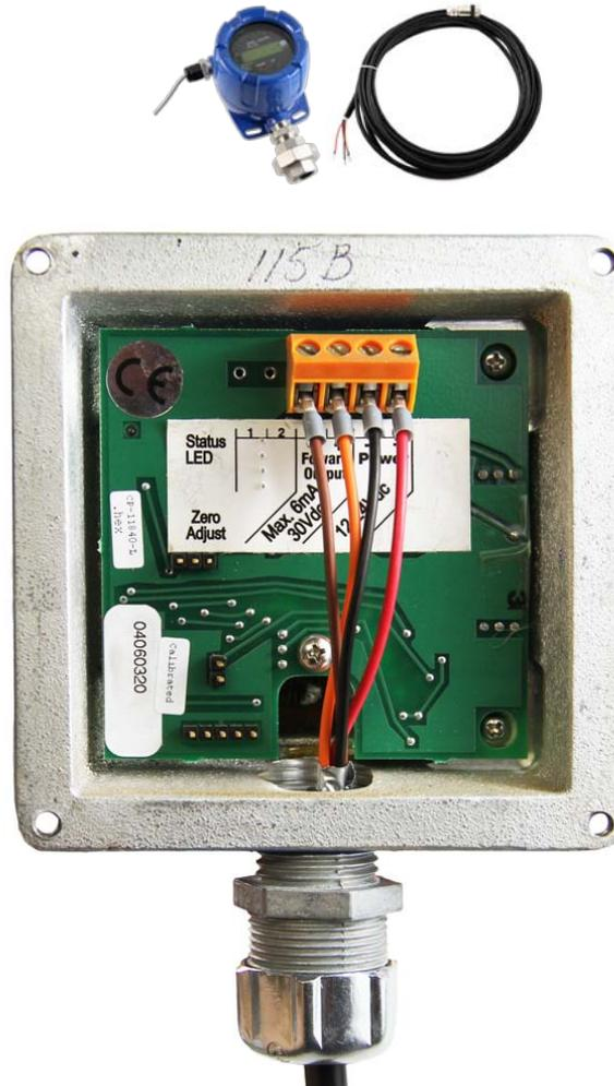
Open the lid which is held down with 4x machine screws and loosen the cable gland. Undo the currently installed cable from the screw terminals and slide it out.
