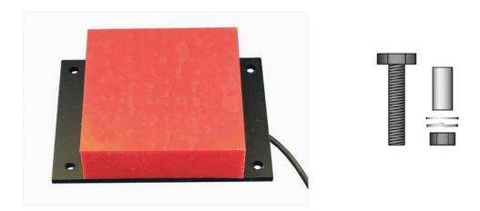
By using bolts and the appropriately sized collar for the thickness of the plate the ANT-IR can be mounted underneath diamond plate. A 5" square hole must be cut out to make room for the antenna face to come through the material as well as 4 holes for the bolts.
