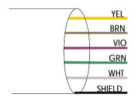
Vs 7-28 VDC RH out 0-1 V 0-100 %RH T out 0-1 V -40 - +60C GND (ground) NC (no connection)
