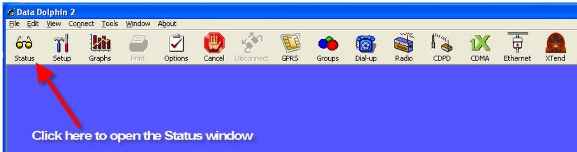
The Status window, accessed in the Data Dolphin software by clicking on the Status button on the toolbar, gives the user a live update of the measured values on the inputs of the datalogger. A datalogger can connect to a computer with the Data Dolphin software either remotely (with a wireless modem) or directly via a serial port connection.
