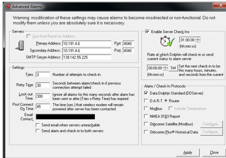
Press **Configure** from the Alarms tab to bring up the advanced alarm window where you can set the regular check in rate and protocols. Typical checks in rates are 4-6 hours, and Data Dolphin Standard should be enabled when a cellular modem is installed for most applications.
