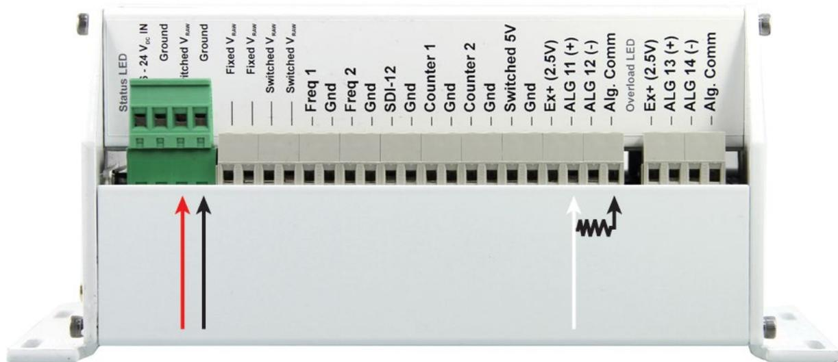
For a three wire 4-20mA sensor the V+ or V DC is connected to Switched Vraw and the V- or GND is connected to Ground. The signal output is connected to ALG 11 and a precision 100 ohm shunt resistor is tied between the input and Alg. Comm.
