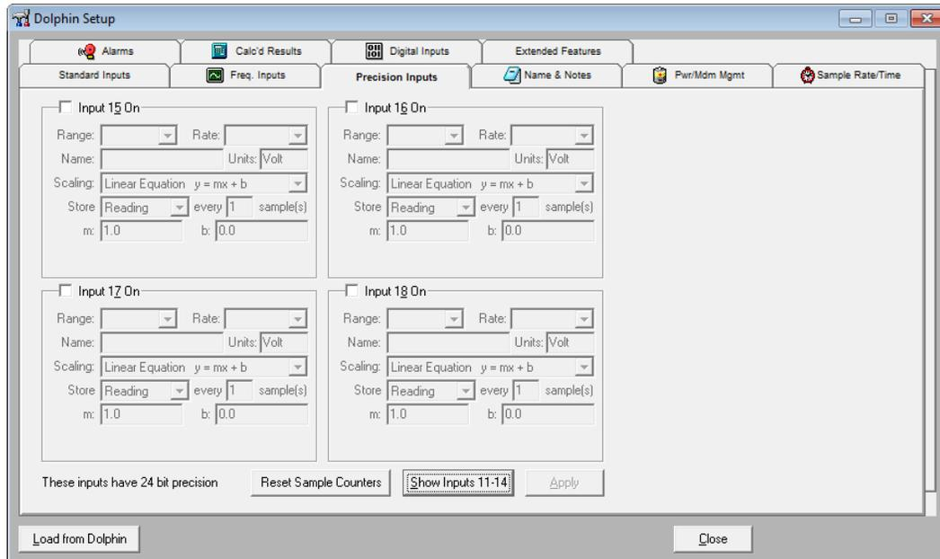
Precision Analog Inputs 11 through 18 have 24 bit precision. These are available on the DD-400 and will most likely be your most used inputs. They can also be configured as differentials with 11 and 12, 13 and 14, 15 and 16, and 17 and 18 being the pairs.
