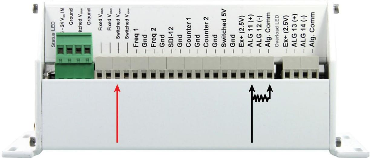
For a two wire 4-20mA sensor the V+ or V DC is connected to Switched Vraw and the V- or GND is connected to ALG 11 and a precision 100 ohm shunt resistor is tied between the input and Alg. Comm.
