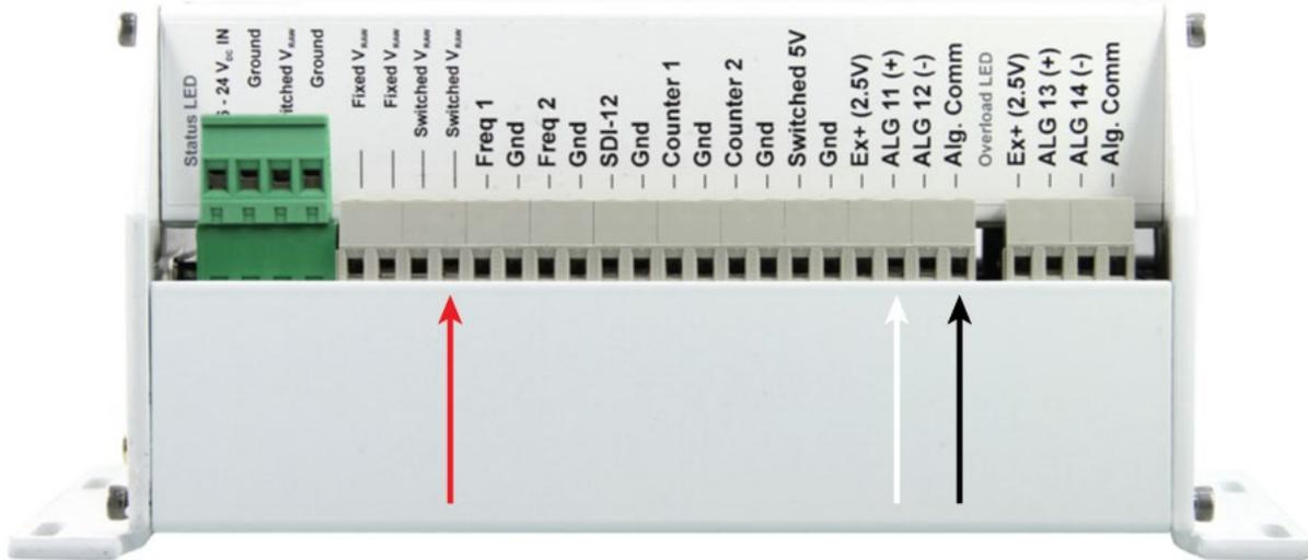
Connect the wires from your sensor to the data logger as shown. The colors shown here are suggested, but may not match your device exactly. Power is connected to the Switched Vraw output and Ground with the output from the sensor going into ALG 11.
