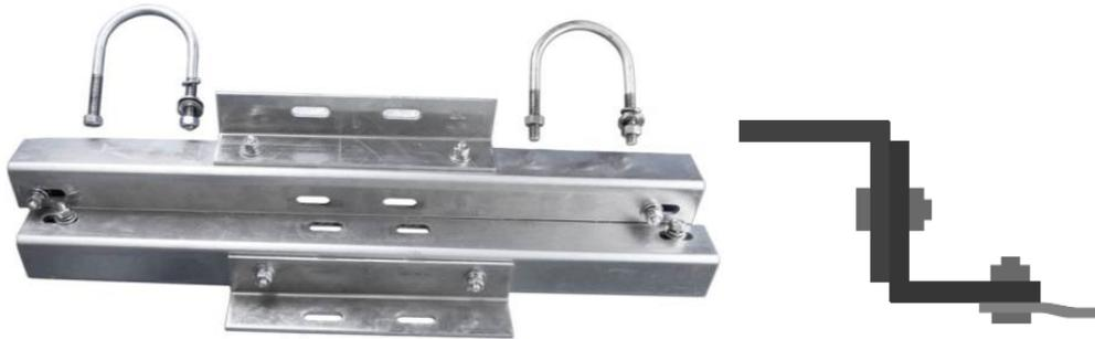
Find the U-Bolts that will attach to the brackets on the fibreglass box. The same type of U-Bolts will also be used to mount the solar panel. Bushings may be necessary on the U-Bolt to clamp tightly to the mast. Newer bracket assemblies are slotted to allow different U Bolt sizes.
