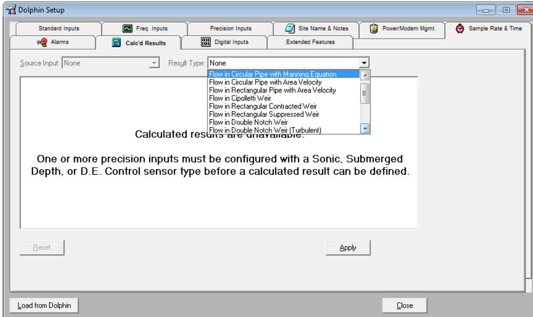
If you have enabled one of your Precision Inputs accordingly one can use calculated results to convert Submerged Depth to a flow rate and total volume using the appropriate calculation from the drop down.
