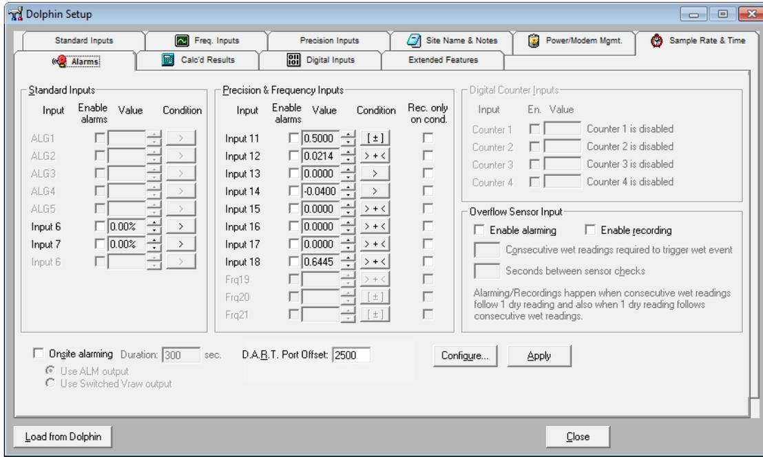
These alarms will watch the Precision Inputs for values that meet certain conditions. When an alarm is triggered this will force the data logger to contact the server if there is telemetry enabled send e-mail and/or SMS notifications.
