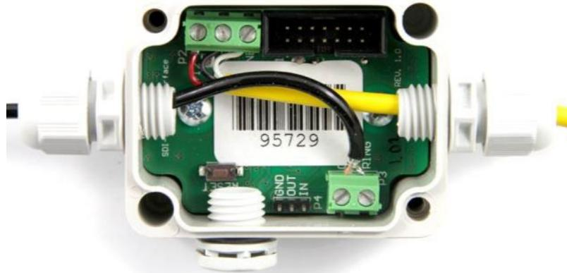
Strip the wire jacket off and twist the shield together to form a pin and tin it with solder. Tin the center wire as well. The yellow jacket wire will provide the power and SDI-12 signal connections to the DD-400. Verify inside the DCX that the red is in +12, black is GND, and white in LINE.
