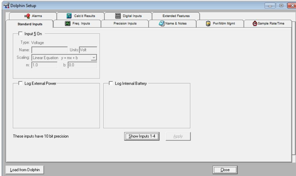
The Data Dolphin data logger can also record its external power source voltage in order to monitor battery levels. Internal Battery provides the voltage reading for the Switched 5V terminal for sensors that need 5V excitation.
