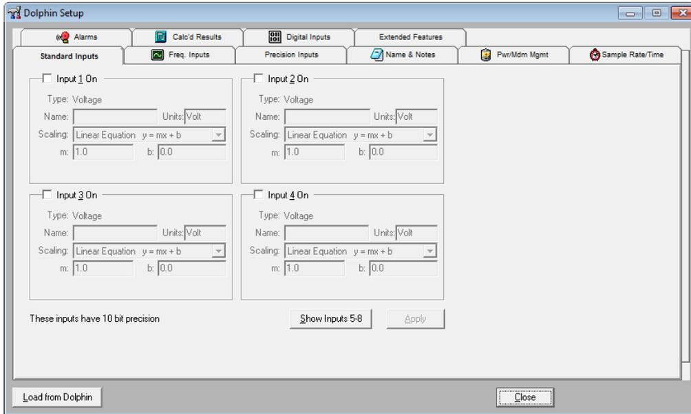
In the DD-400 and DD-200 these are 10 bit analog inputs. Linear equation scaling can be set, or if you are using a thermistor the drop down for Scaling can automatically set the coefficients appropriately.
