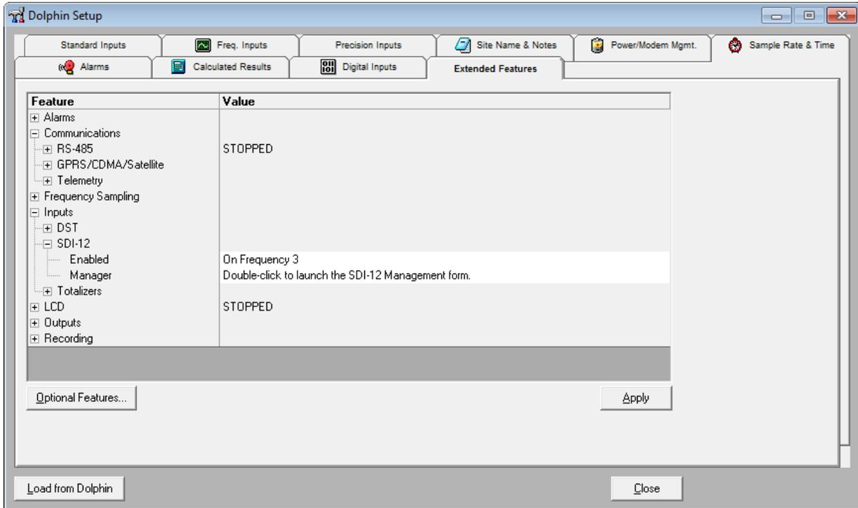
SDI-12 functionality can be enabled from the Extended Features on your Frequency 3 input. This is now the default for all DD-400 data loggers with firmware greater than 166.0.
