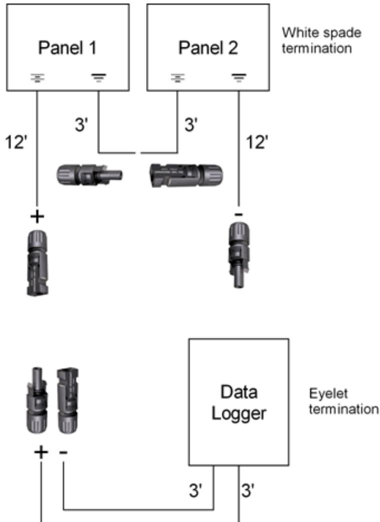
If your system is 24V powered then you will have two panels in series. The panels mount side by side on the same bracket. Mount and connect Type 1 and Type 2 panels together with the short cables. The longer MC4 cables go into the DLS-400 enclosure.
