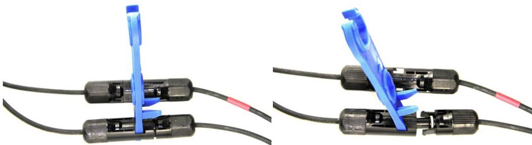
Simply push the tool into the slots and twist it to release.
