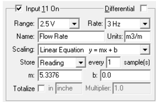
The pulse counter input must also be set with an m that corresponds to the Relay 1 Pulse value. In the above testing it was set to 0.250 m<sup>3</sup> per pulse. These values will depend on the ID of your pipe so ensure you calculate this for each station.
