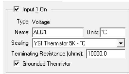
As an example Input 1 has a 5K thermistor with a 10K ohm terminated resistor. With this setup the thermistor is wired between Input 1 and Ground, and the termination resistor is wired between Ex+ (2.5V) and Input 1.
