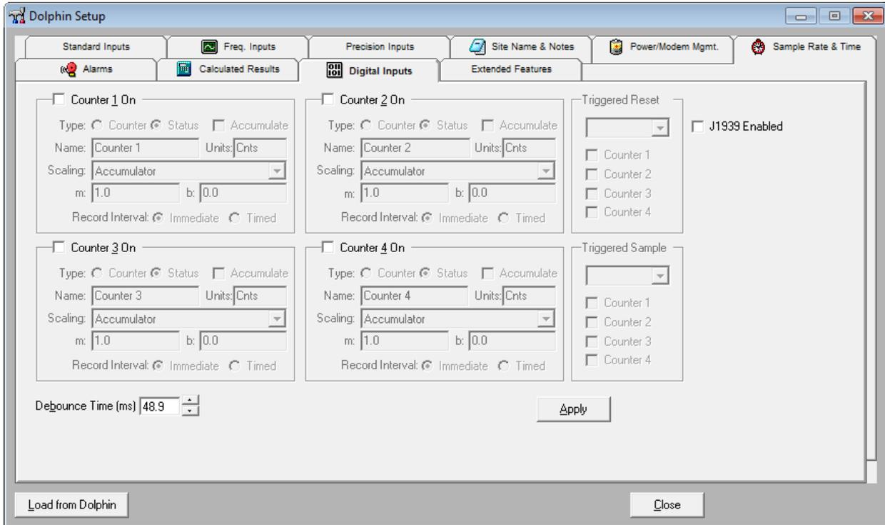
Counter Inputs can either be configured as a status or counter. Recording can also be based on the data logger sample rate or can be done at the moment the counter receives a signal.
