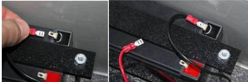
Next connect the **red** wire to the **red** positive terminal on the battery and push it all the way on.
