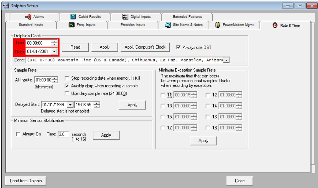
This is the tab that initiates the data logging once the Dolphins Clock has been set. You can set the time zone, and whether or not to always use DST. The time and date will be highlighted in red if the data logger is NOT currently logging with a correctly set clock.
