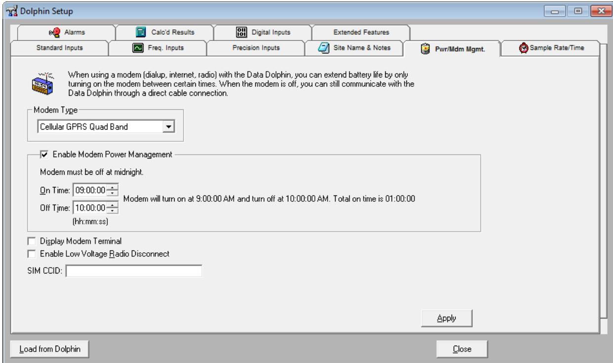
This tab lets you select the telemetry that is installed in your data logger. If there is none then “None (RS-232 Only)” will be selected.
