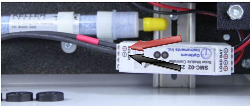
Disconnect the solar panel and check that the system runs on just battery power as well in the case of a battery not holding any charge and in need of replacement.
