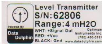
The wire colors and connection is listed on this label. See the section “Level Transmitter –Analog output” wiring section in this manual.
