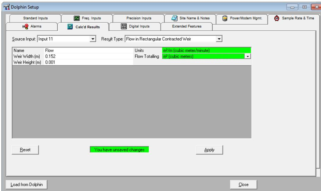
For example a rectangular contracted weir is selected and output will be in m<sup>3</sup>/min for flow and cubic meters for total volume.
