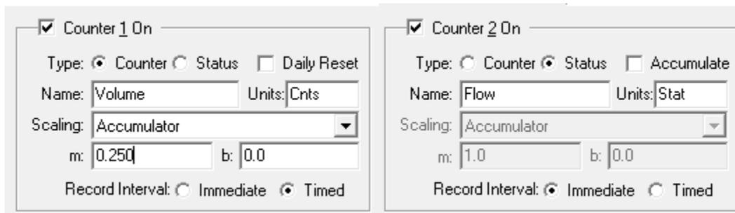
Apply your settings and the pulse and flow rate outputs from the DFM will now be recorded correctly.
