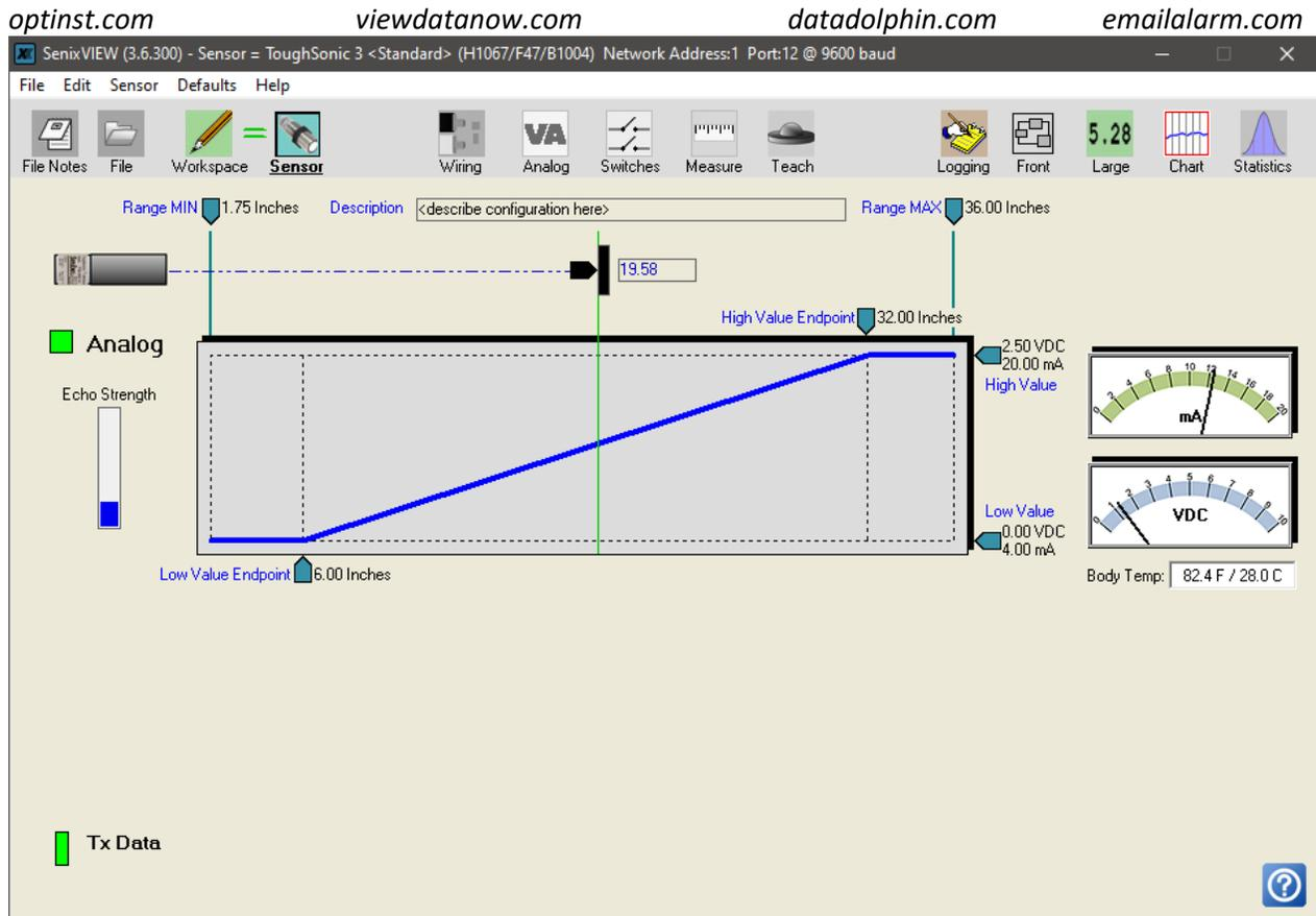
Scaling of the sensor should be set such that the maximum expected range outputs 2.50V and the minimum expected range outputs 0.00V
