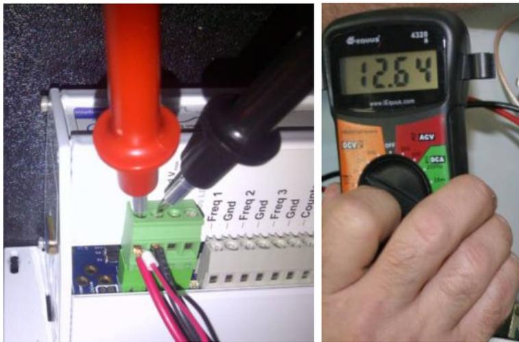
Measure the voltage at the solar panel connection. You should see between 14 VDC to 21 VDC if the sun is shining.
