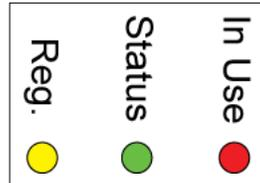
The Yellow Registration LED on the side of the DD-400 should also be on steady and will eventually start flashing. A flashing yellow LED means that we have found a cellular service provider and have successfully signed in with a valid account.
