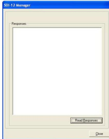
To read the attached SDI-12 sensors current values, press the “Read Responses” button. This will tell the data logger to poll the SDI-12 device for its current readings. Every time you press the button the progress will be shown if there is a measurement time remaining.
